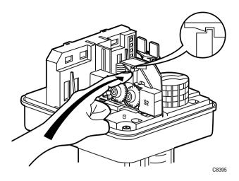
Fig. 3. Securing auxiliary switch assembly.
